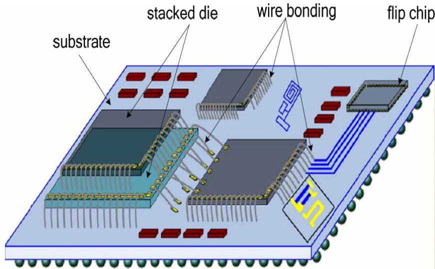
Fig. An example of IC package.
