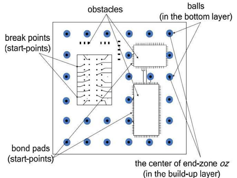
Fig. Substrate routing graph (SRG) in a signal layer
