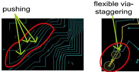
Fig. 16. Partial substrate routing based on dynamic pushing and flexible via staggering.
