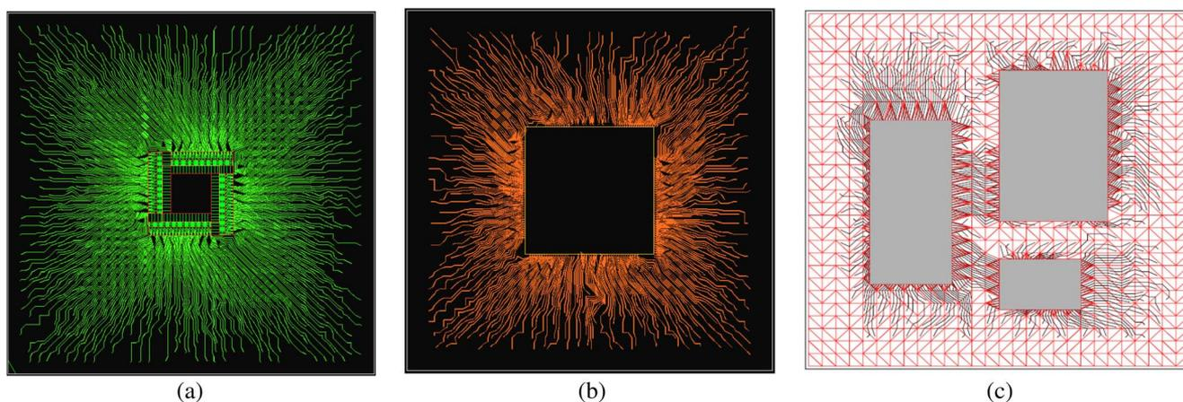
Fig. 15. Topological routing results on a buildup layer. (a) Case 3. (b) Case 4. (c) Case 8.
