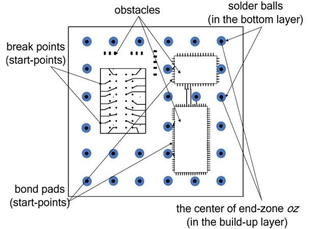
Fig. 3. SRG in a buildup layer.
