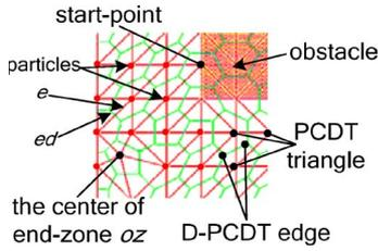
Fig. 4. Partial PCDT and D-PCDT.
