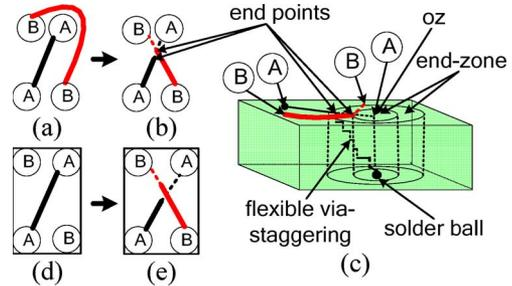
Fig. 11. Comparison between fixed end-point [(a) Detour and (d) Unroutable] and flexible via-staggering [(b) Nondetour, (c) 3-D description, and (e) Routable].
