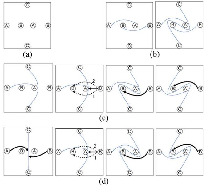
Fig. 8. Example of net ordering. (a) Nets initial location. (b) Net order (A, B)–C and routing. (c) Net order A–C–B and routing. (d) Net order C–(A, B) and routing. Only this work can obtain routing (c) and (d).
