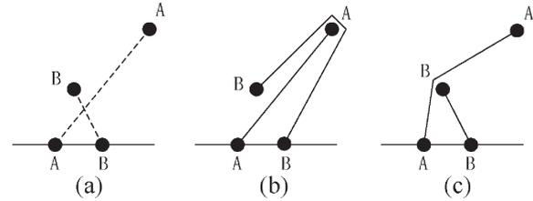
Fig. 10. Different routing results between the “traditional rip-up and reroute” and “dynamic pushing.” (a) Given nets. (b) Routing result by the traditional rip-up and reroute. (c) Routing result by dynamic pushing.
