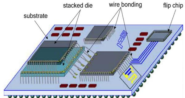
Fig. 1. Example of an IC package.
