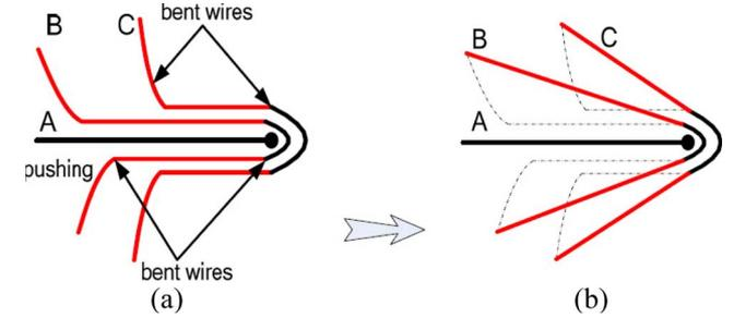
Fig. 14. (a) Bent. (b) Stretch.
