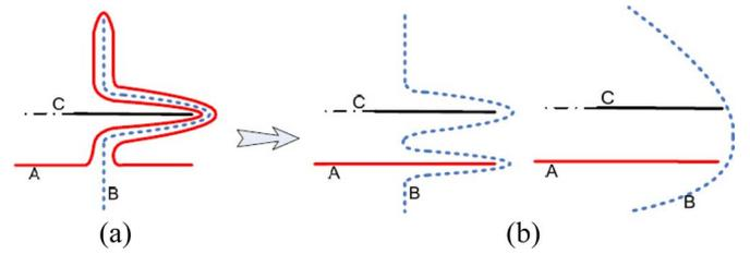
Fig. 13. Reordering and finding a better solution. (a) Net A is pushed twice. (b) Better solution.
