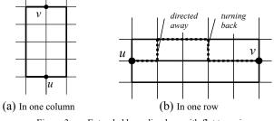
Figure 3. Extended bounding box with flat two pins
